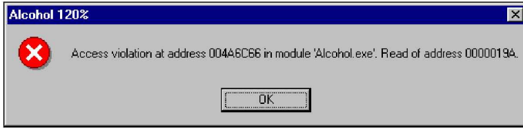
Fig. 6.16. Response of Alcohol 120% to an attempt of burn the CD image with only track number zero inside the first session
